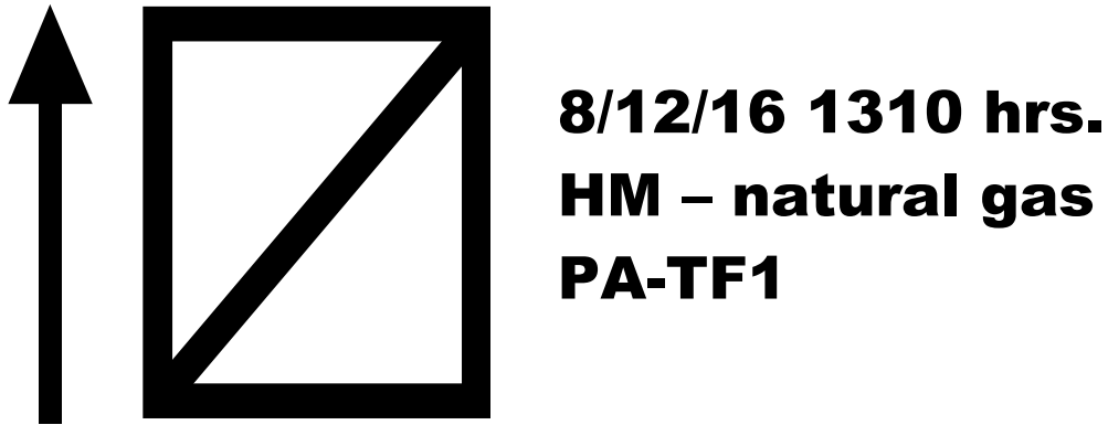
FIGURE 9: Structure/Hazards Evaluation Marking Indicating a Medium Risk Building
